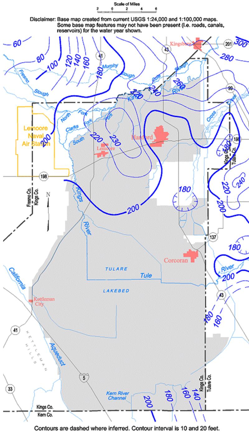
**E 29** Unconfined aquifer groundwater contour map, Tulare Lake groundwater basin, Spring 1984.
