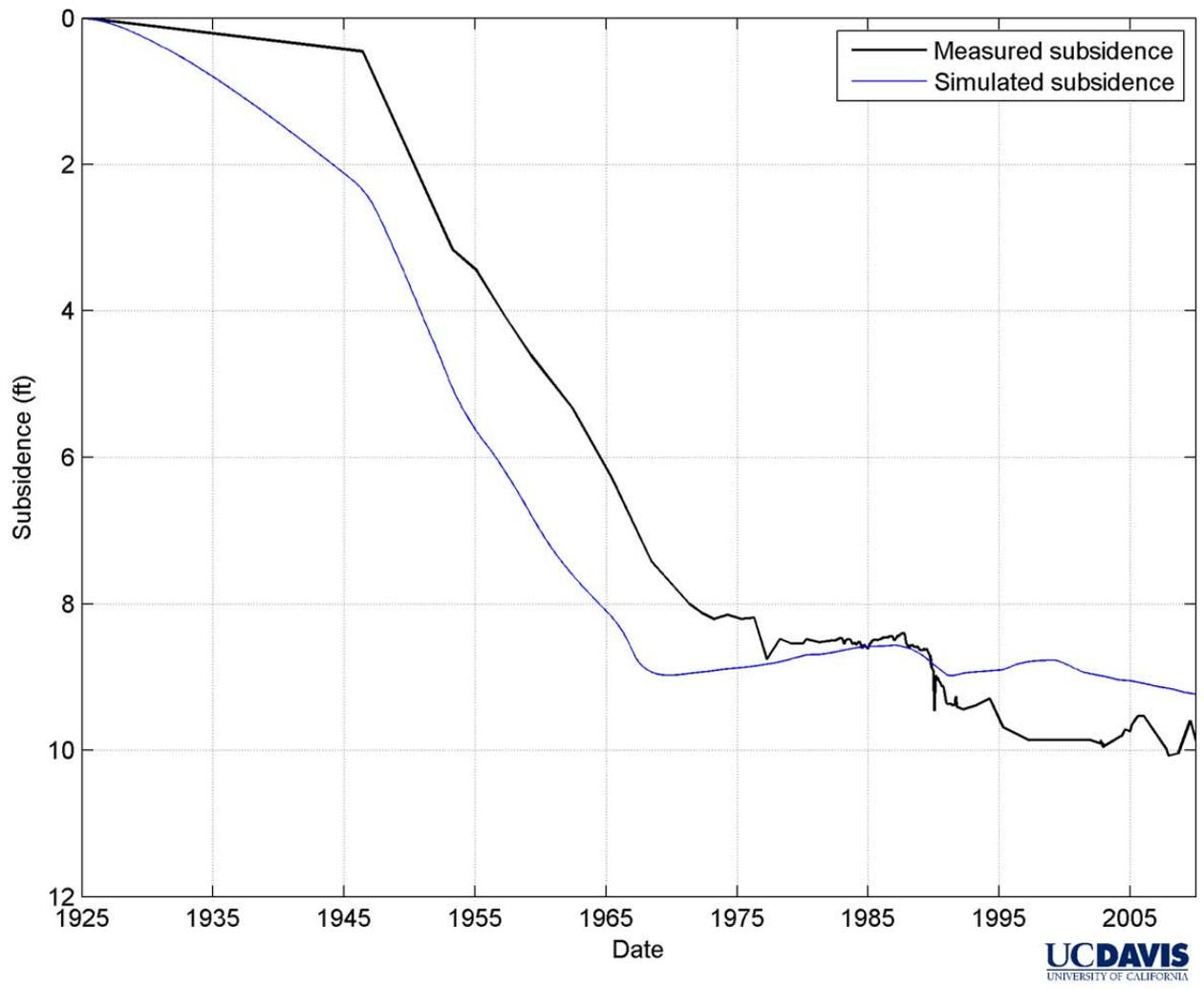
**Figure 61** Simulated and measured subsidence results at NASL
