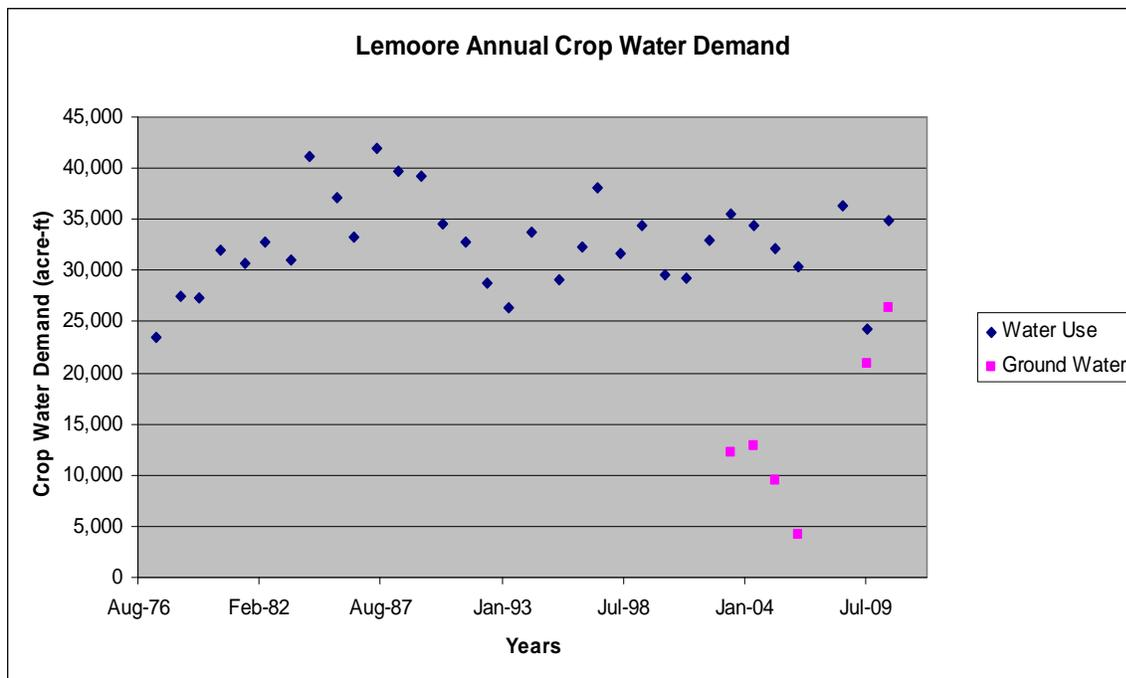
**Figure 6** Annual applied water demand for irrigating the crops at NASL from 1974 through 2010.
