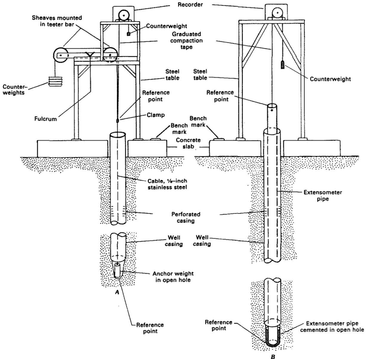
**Figure 49** Typical extensometer construction (Riley, 1984).
