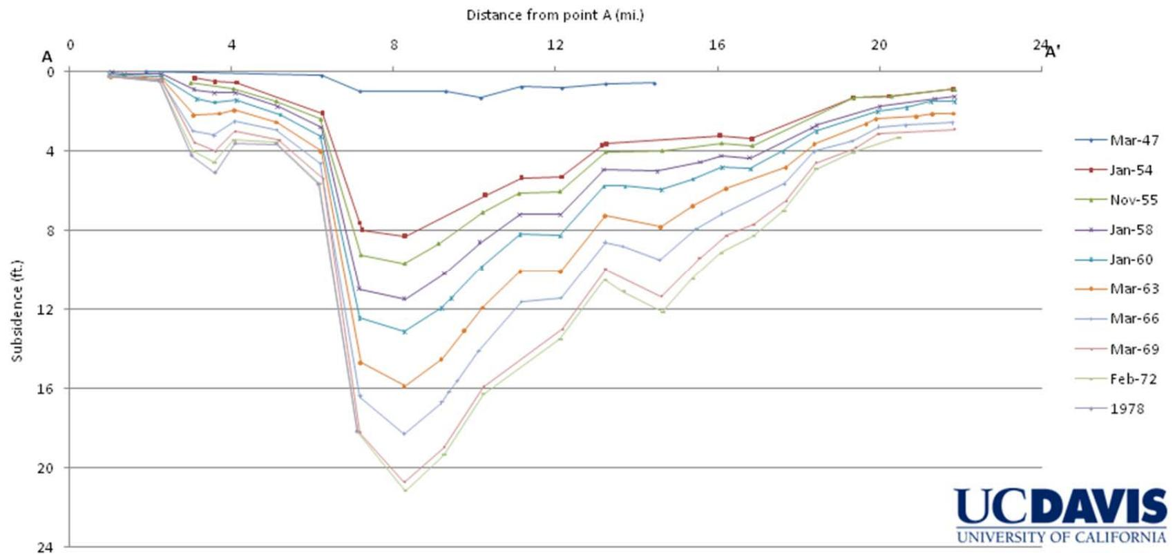
Figure 55 Subsidence profile line A-A' (digitized version of H-H' shown in Figure 52).
