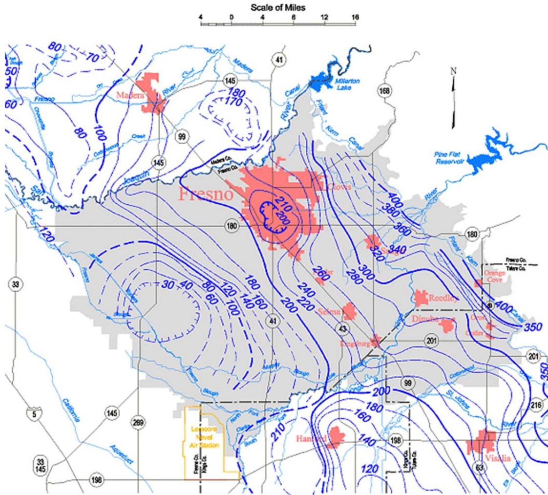
Contours are dashed where inferred. Contour interval is 10, 20 and 50 feet.
