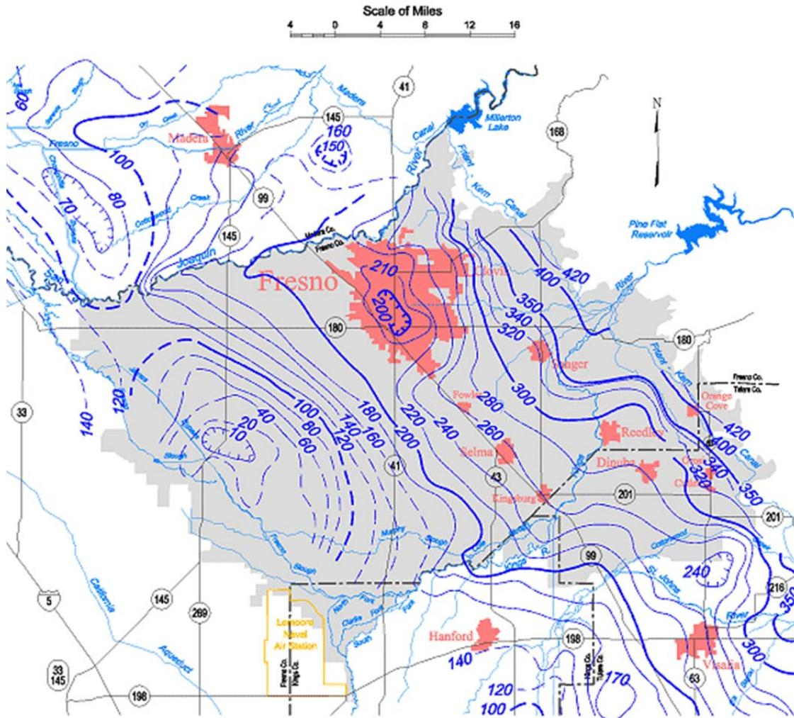
E 12 Unconfined aquifer groundwater contour map, Kings groundwater basin, Spring 1994.
