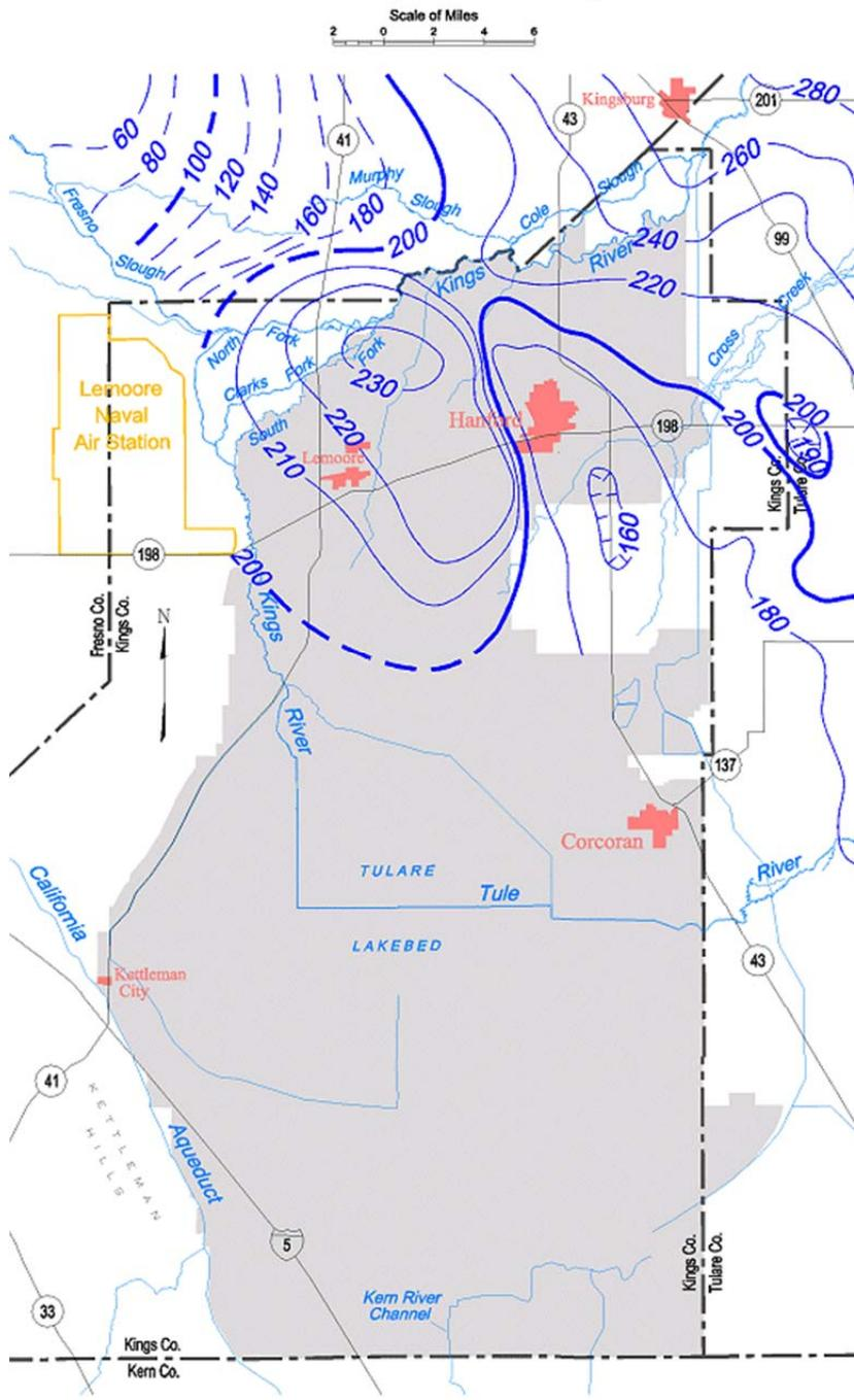
**E 30** Unconfined aquifer groundwater contour map, Tulare Lake groundwater basin, Spring 1989.
