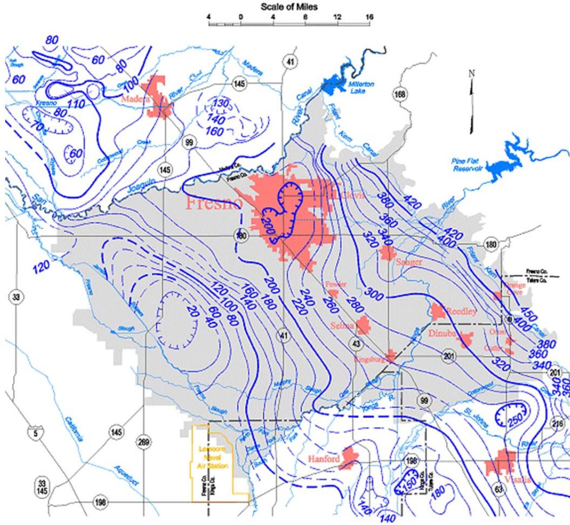
E 20 Unconfined aquifer groundwater contour map, Kings groundwater basin, Spring 2002.
