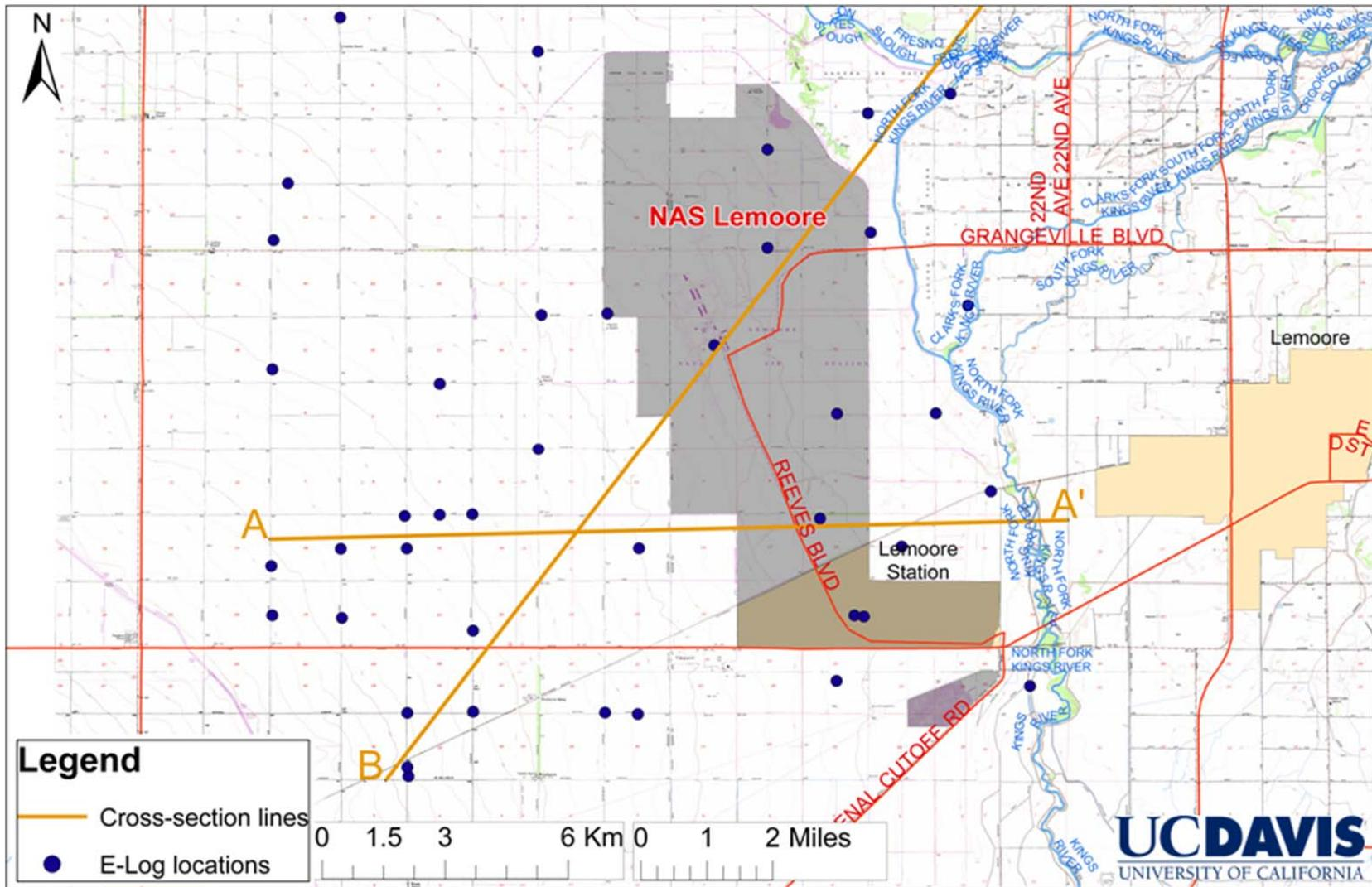
Figure 21 NASL geologic cross-section location (orange lines) and location of E-logs selected for analysis (blue dots).
