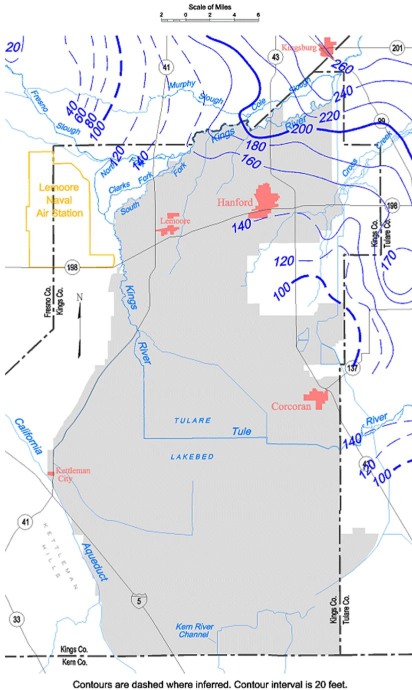
**E 35** Unconfined aquifer groundwater contour map, Tulare Lake groundwater basin, Spring 1994.
