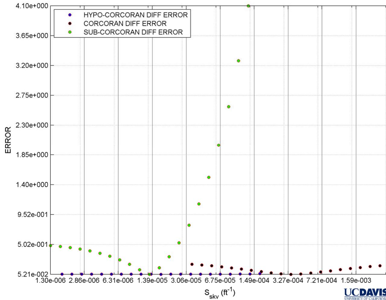
**Figure 73** Diffusivity error distribution between measured and simulated parameter values. Hypo-Corcoran, Corcoran and sub-Corcoran  $S'_{ske}$  values are  $4.00 \times 10^{-6}$ ,  $4.00 \times 10^{-6}$  and  $1.20 \times 10^{-6} \text{ ft}^{-1}$ , respectively.
