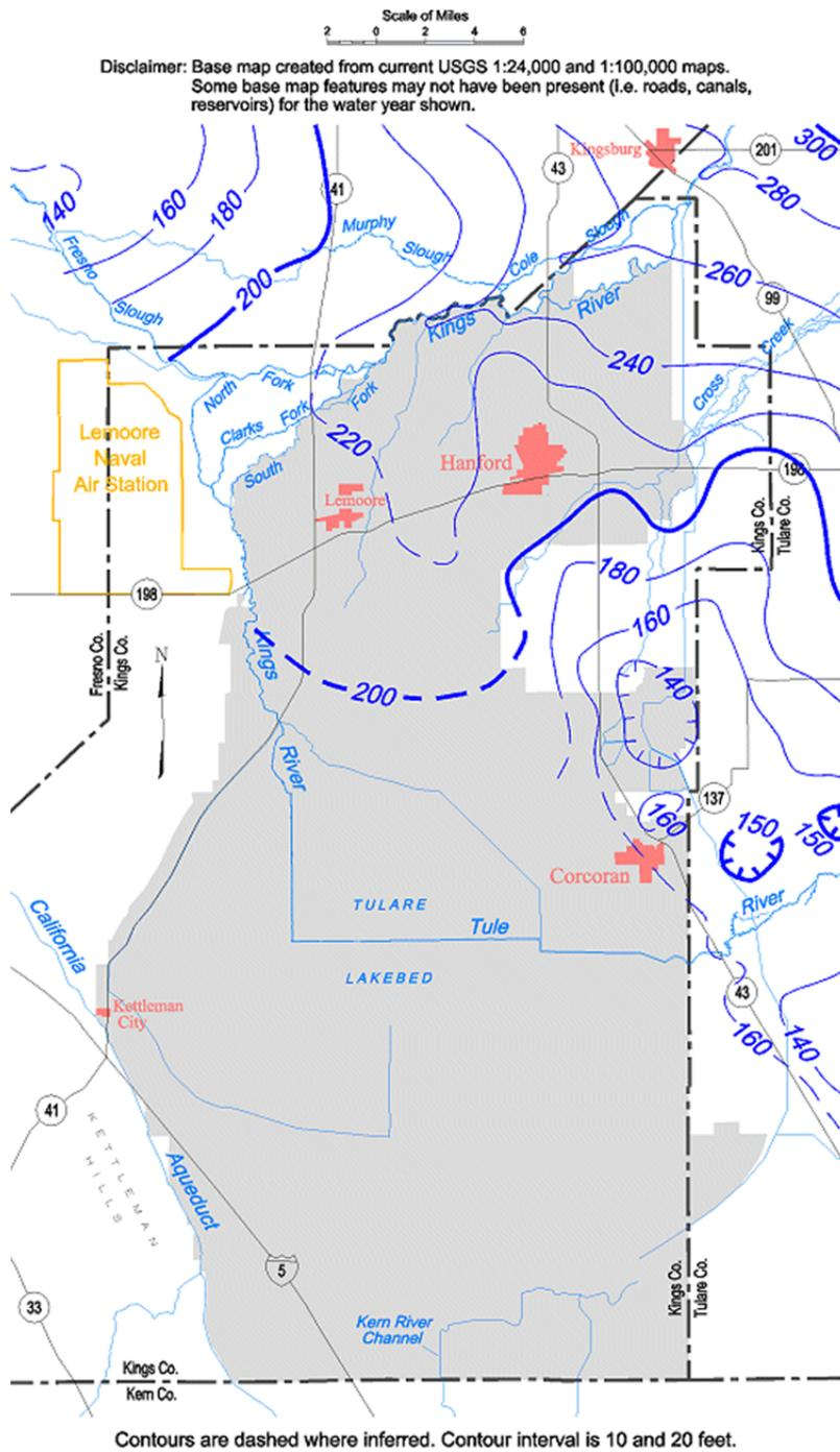
**E 24** Unconfined aquifer groundwater contour map, Tulare Lake groundwater basin, Spring 1958.
