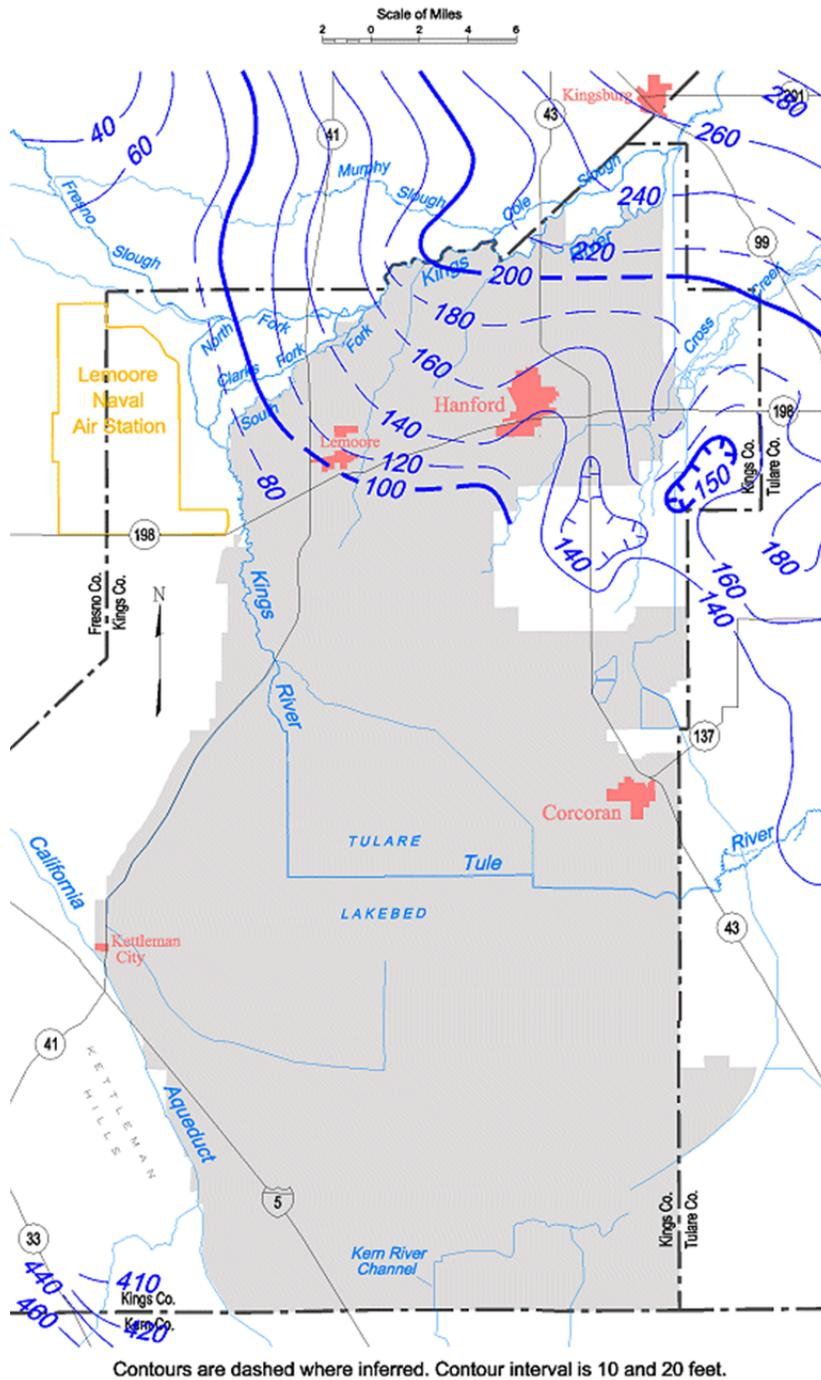
**E 43** Unconfined aquifer groundwater contour map, Tulare Lake groundwater basin, Spring 2002.
