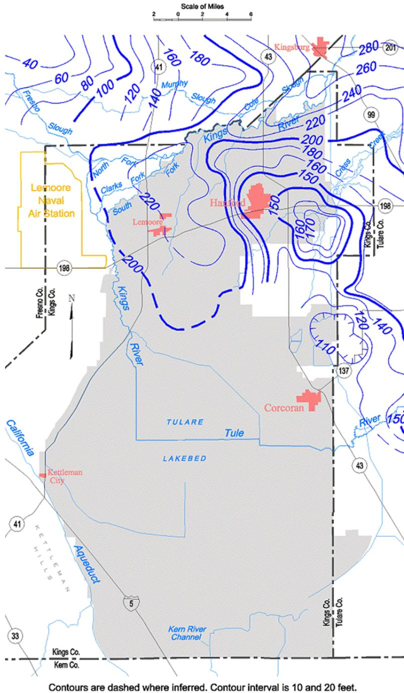
**E 38** Unconfined aquifer groundwater contour map, Tulare Lake groundwater basin, Spring 1997.
