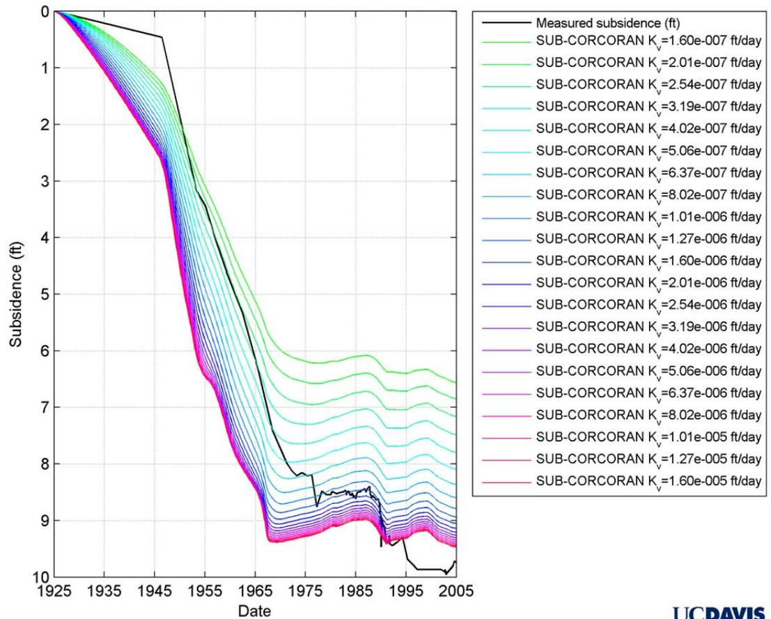
**Figure 72** Sub-Corcoran vertical hydraulic conductivity compaction trajectories. Hypo-Corcoran and Corcoran  $K'_v$  values are  $7.10E-06$  and  $1.20E-05$  ft/day, respectively. Hypo-Corcoran, Corcoran and sub-Corcoran  $S'_{skv}$  values are  $1.70E-05$ ,  $3.50E-04$  and  $1.30E-05$   $\text{ft}^{-1}$ , respectively. Hypo-Corcoran, Corcoran and sub-Corcoran  $S'_{ske}$  values are  $4.00E-06$ ,  $4.00E-06$  and  $1.20E-06$   $\text{ft}^{-1}$ , respectively.
