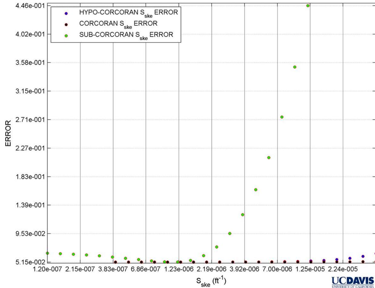
**Figure 69** Elastic skeletal specific storage error distribution between measured and simulated parameter values. Hypo-Corcoran, Corcoran and sub-Corcoran  $K'_v$  values are 7.10E-06, 1.20E-05 and 1.60E-06 ft/day, respectively. Hypo-Corcoran, Corcoran and sub-Corcoran  $S'_{skv}$  values are 1.70E-05, 3.50E-04 and 1.30E-05  $\text{ft}^{-1}$ , respectively.
