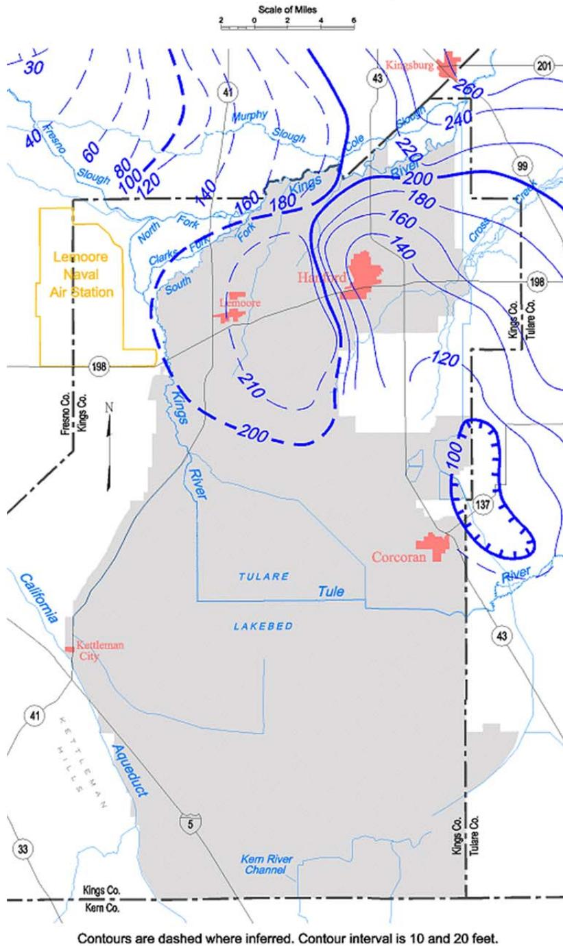
**E 36** Unconfined aquifer groundwater contour map, Tulare Lake groundwater basin, Spring 1995.
