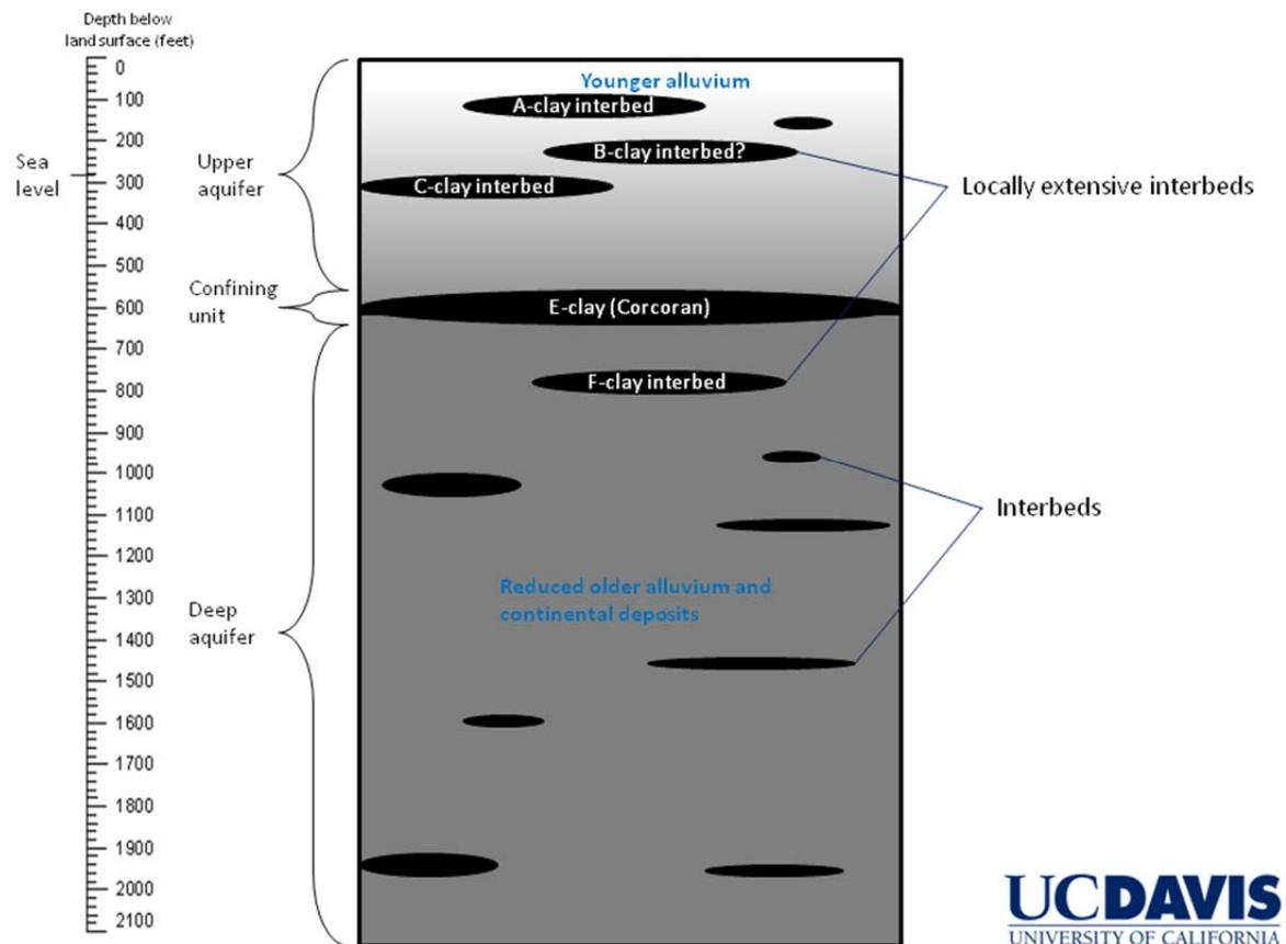
**Figure 24** Simplified study area stratigraphy as presented in several available reports showing upper aquifer that confines with depth due to the A-C-Clay layers, and the deep aquifer.
