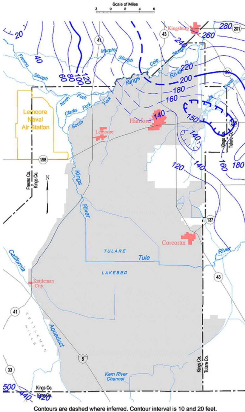
**E 44** Unconfined aquifer groundwater contour map, Tulare Lake groundwater basin, Spring 2003.
