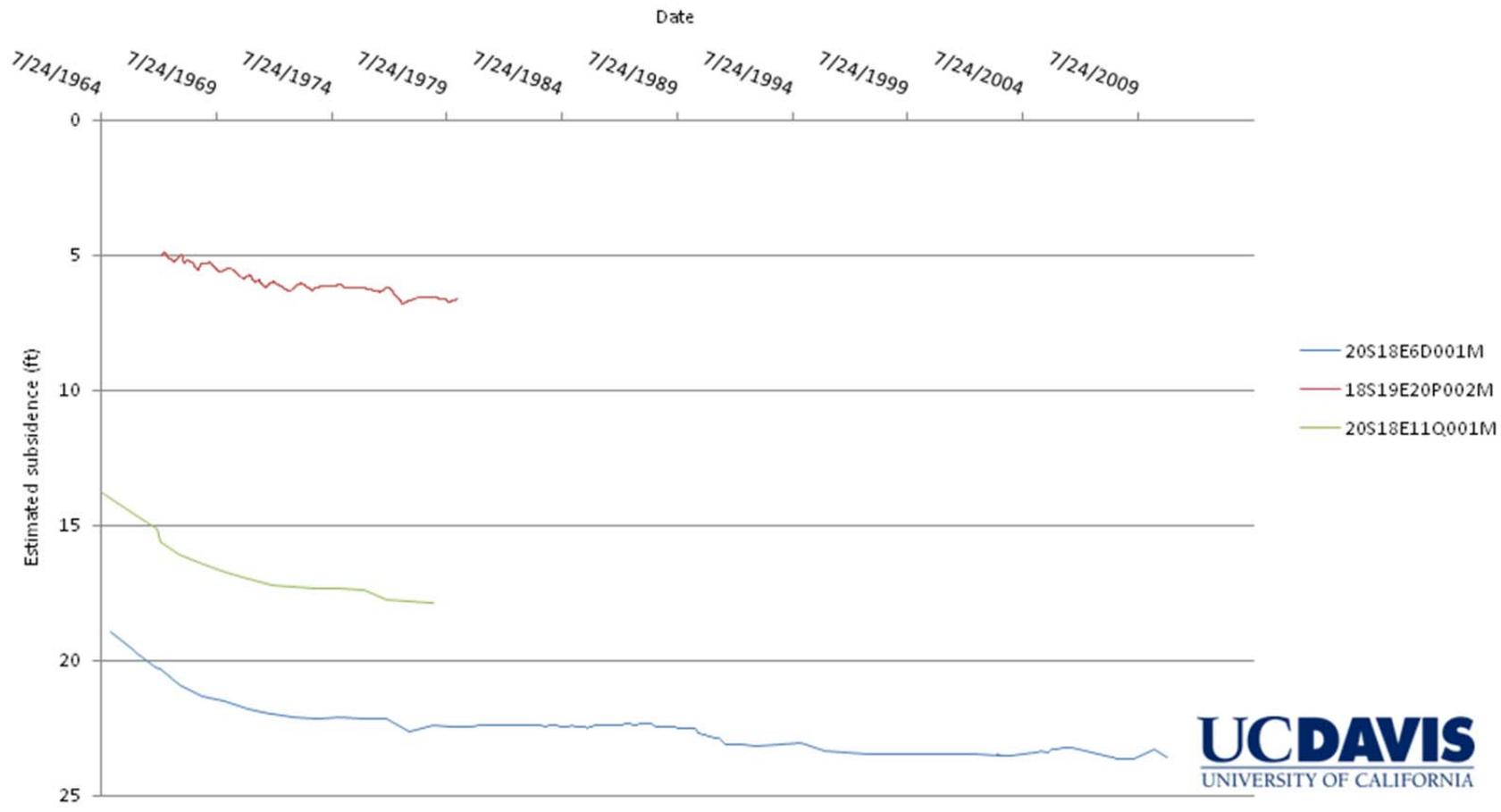
**Figure 57** Estimated compaction at study area extensometers
