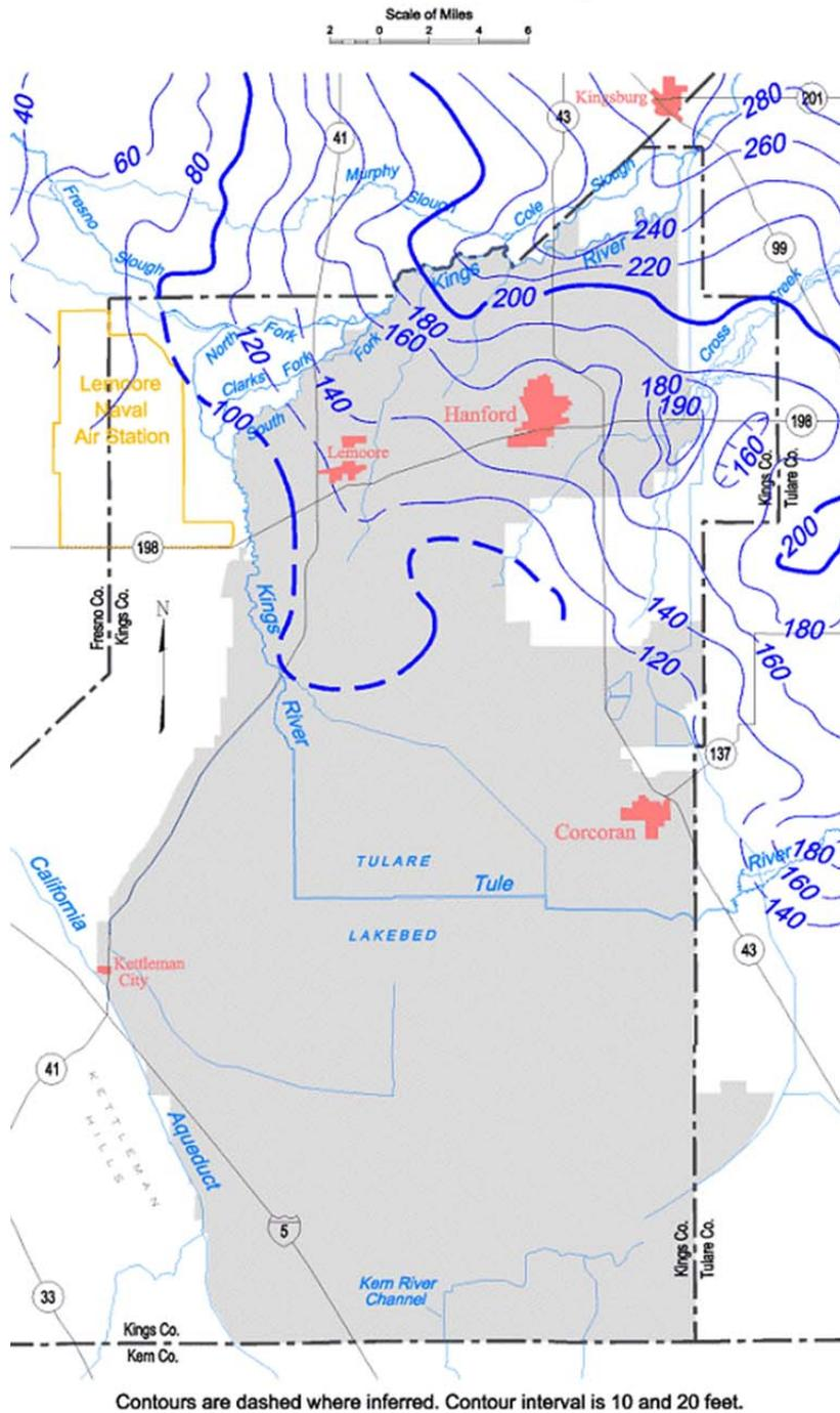
**E 41** Unconfined aquifer groundwater contour map, Tulare Lake groundwater basin, Spring 2000.
