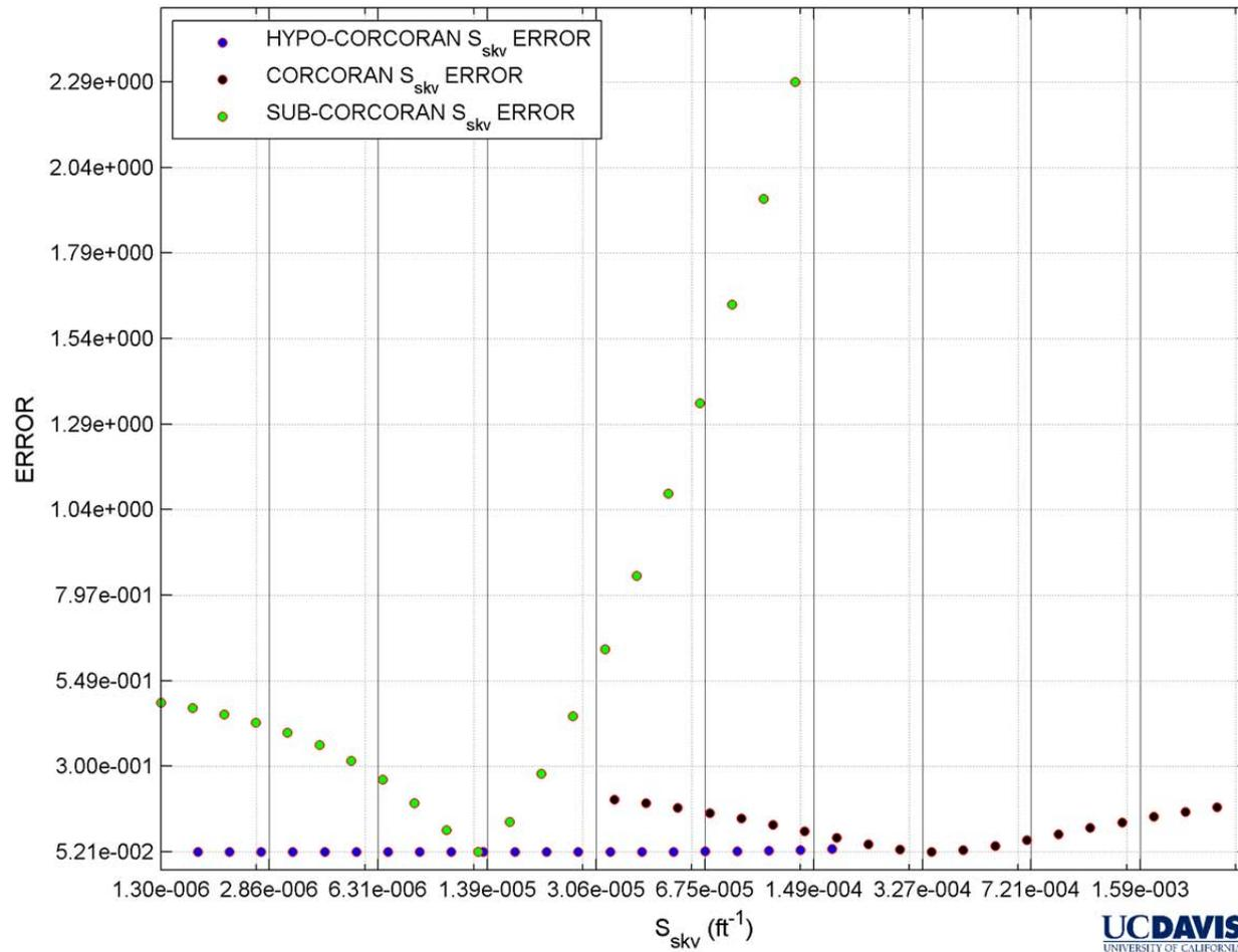
**Figure 67** Inelastic skeletal specific storage error distribution between measured and simulated parameter values. Hypo-Corcoran, Corcoran and sub-Corcoran  $K'_v$  values are 7.10E-06, 1.20E-05 and 1.60E-06 ft/day, respectively. Hypo-Corcoran, Corcoran and sub-Corcoran  $S'_{ske}$  values are 4.00E-06, 4.00E-06 and 1.20E-06 ft<sup>-1</sup>, respectively.
