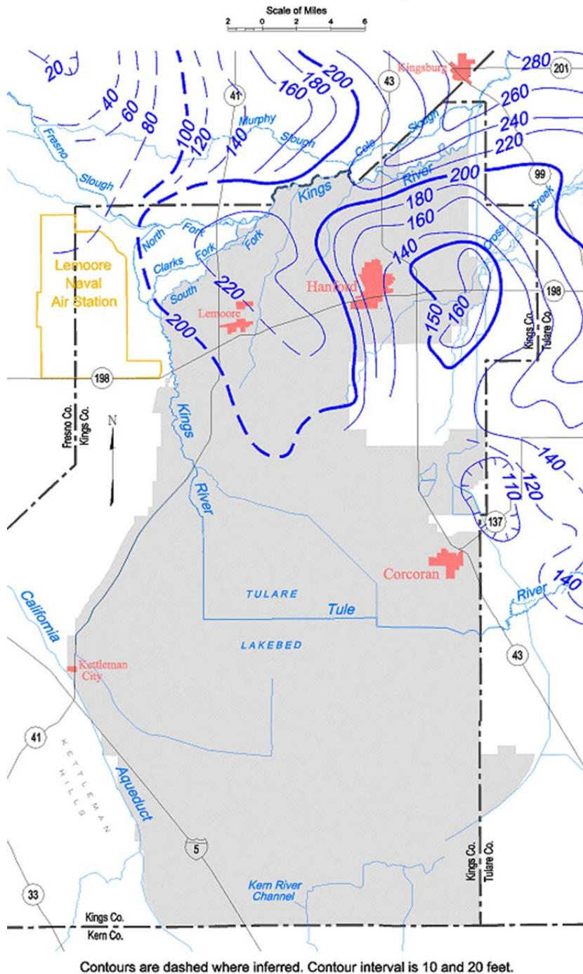
**E 37** Unconfined aquifer groundwater contour map, Tulare Lake groundwater basin, Spring 1996.
