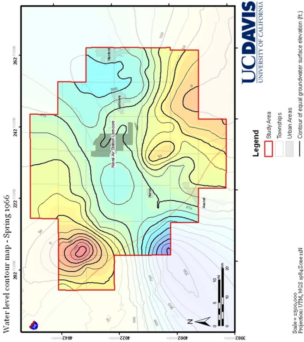
**C 1** Water level contour map for the intermediate and deep aquifer for Spring 1966. Data obtained from the California Department of Water Resources.
