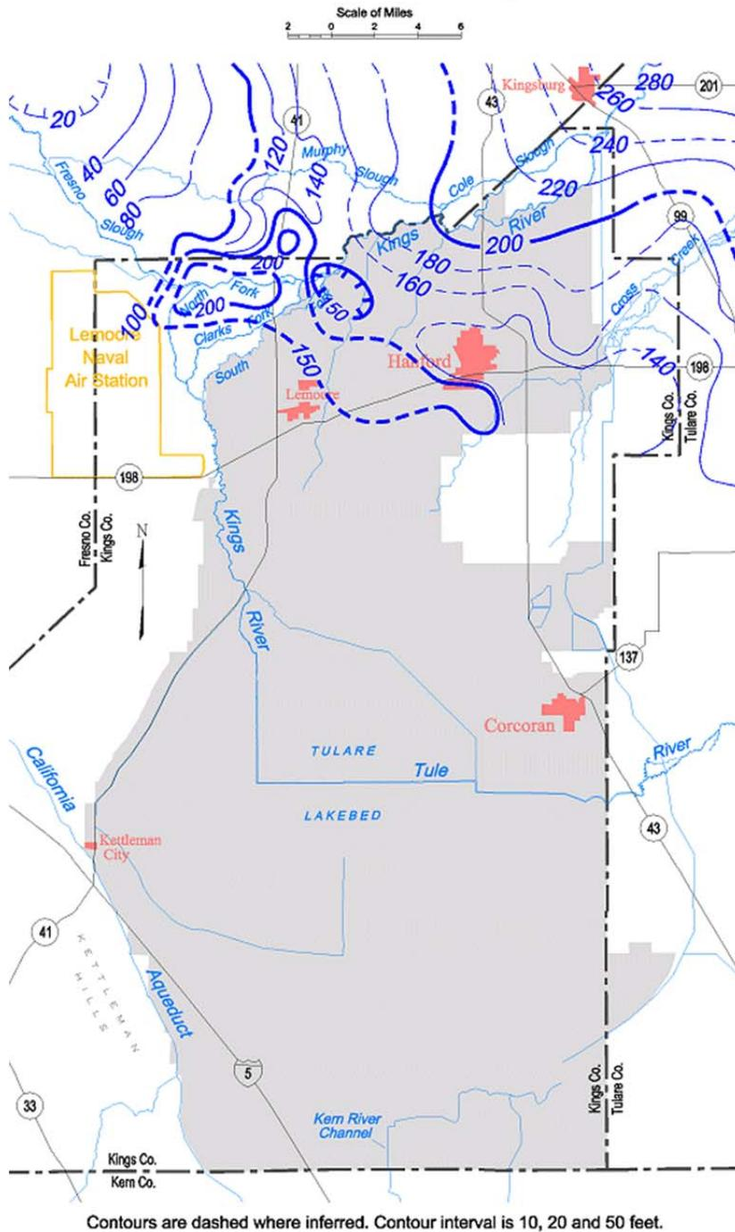
**E 45** Unconfined aquifer groundwater contour map, Tulare Lake groundwater basin, Spring 2004.
