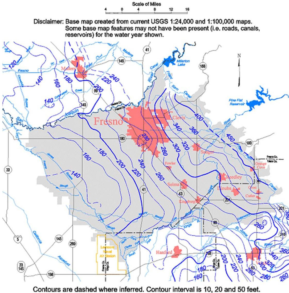
E 1 Unconfined aquifer groundwater contour map, Kings groundwater basin, Spring 1958.
