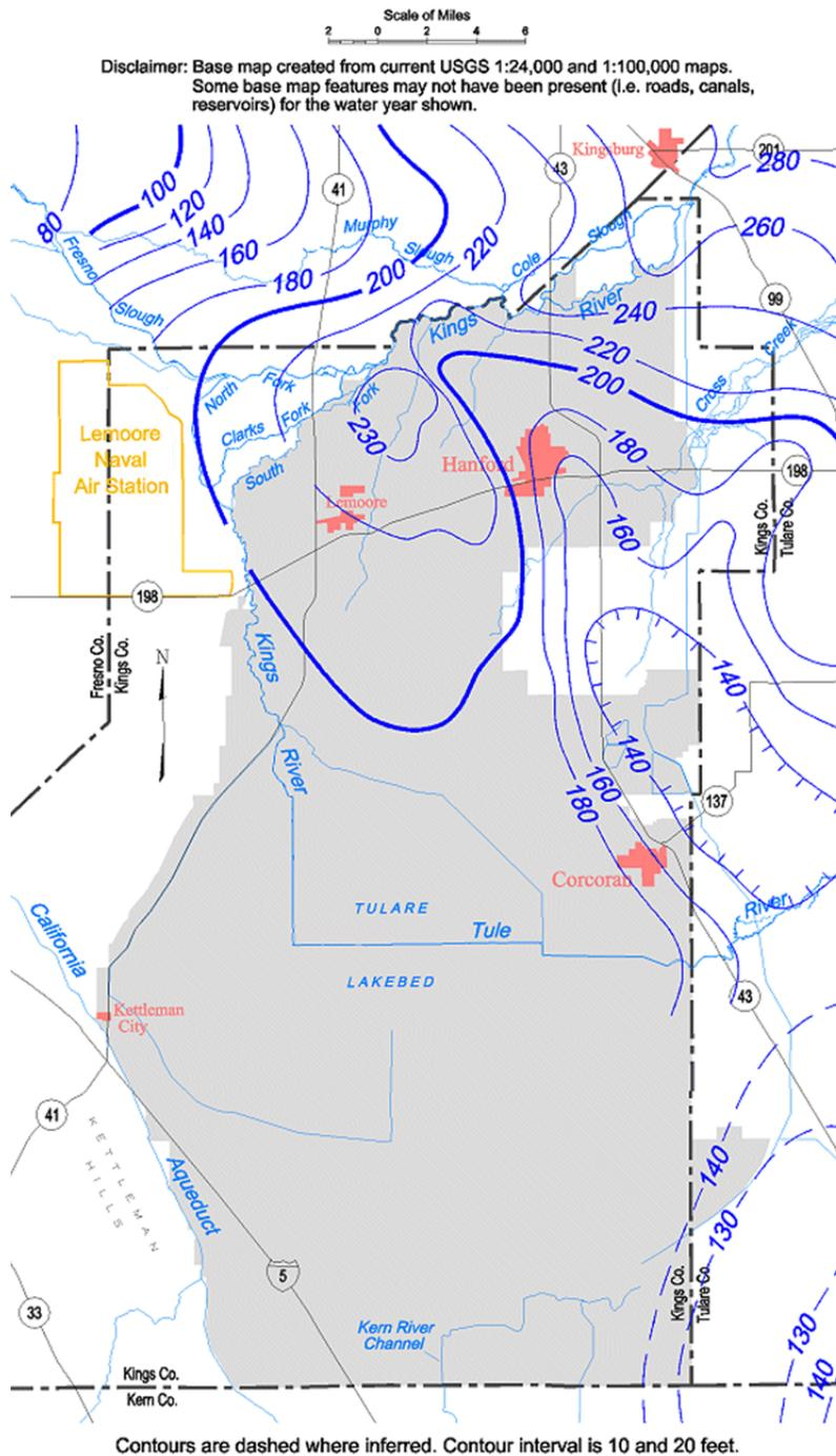
E 26 Unconfined aquifer groundwater contour map, Tulare Lake groundwater basin, Spring 1969.
