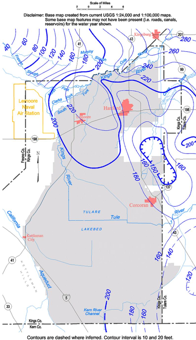
**E 28** Unconfined aquifer groundwater contour map, Tulare Lake groundwater basin, Spring 1976.
