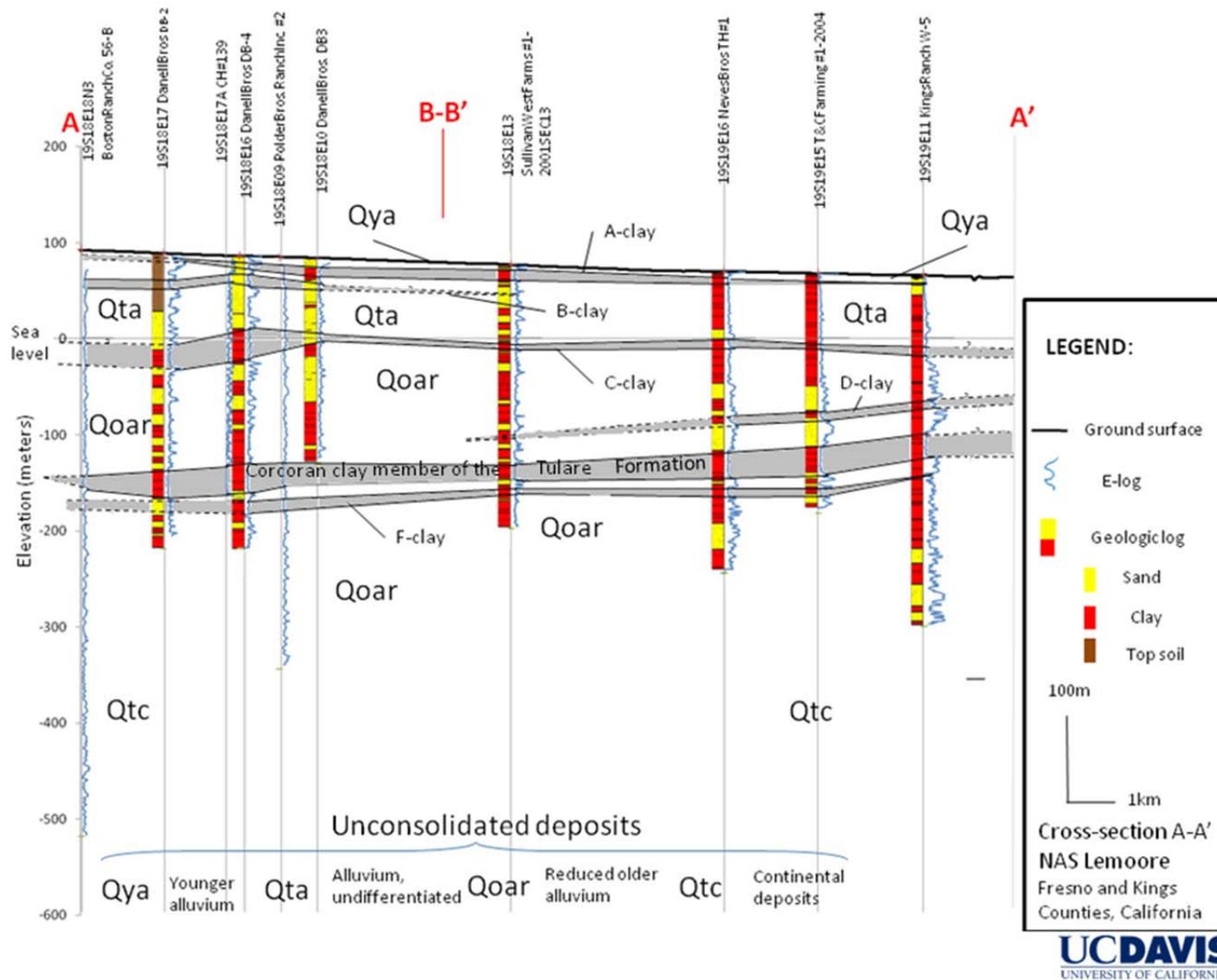
Figure 22 Geologic cross-section A-A' (lines dashed where inferred).
