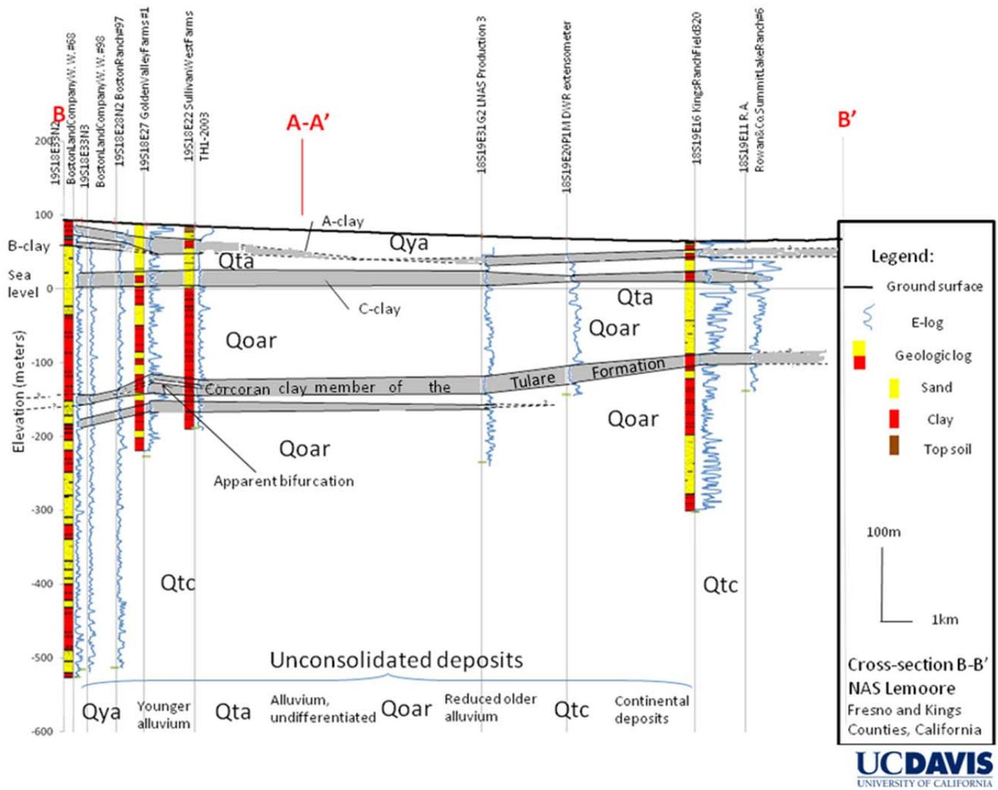
**Figure 23** Geologic cross-section B-B' (lines dashed where inferred).
