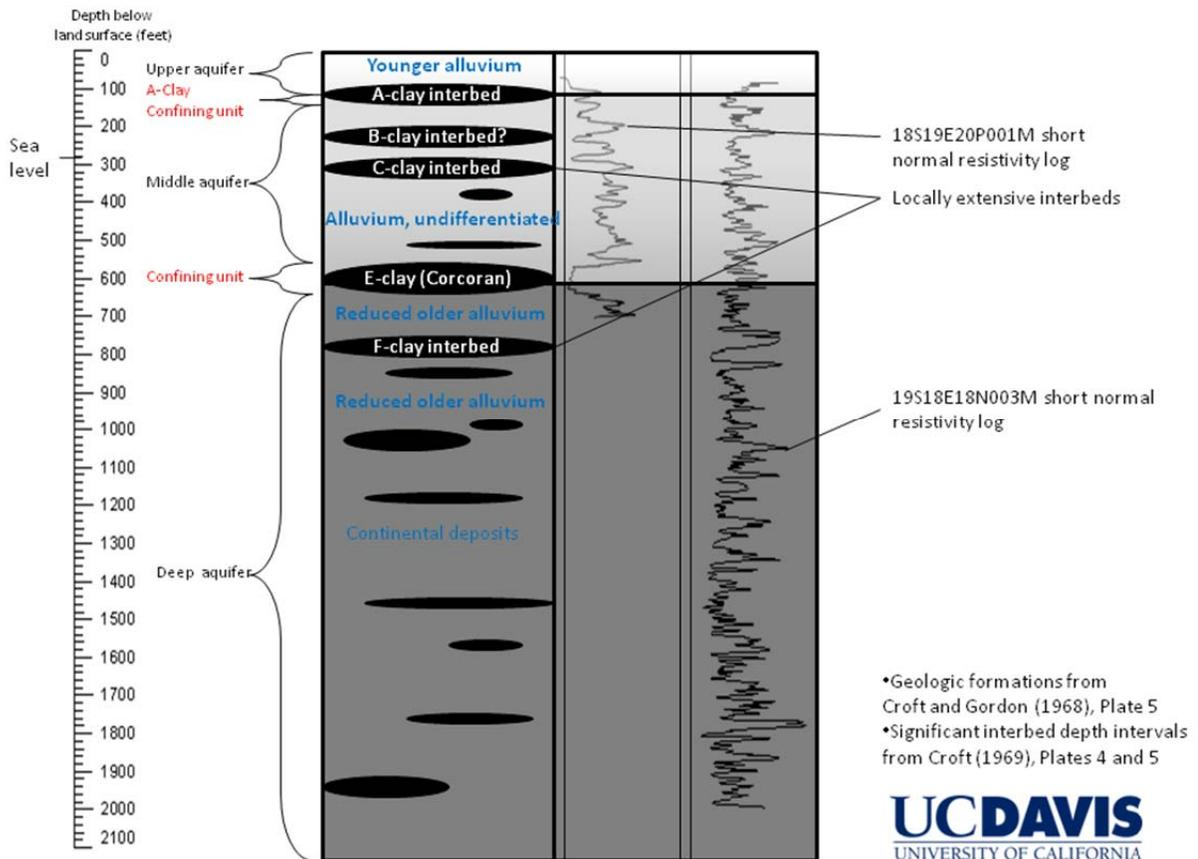
**Figure 25** Detailed study area stratigraphy interpreted from site-specific E-Logs showing upper aquifer above the A-clay confining unit and a middle aquifer that confines with depth due to the B- and C-Clay layers, and the deep aquifer.
