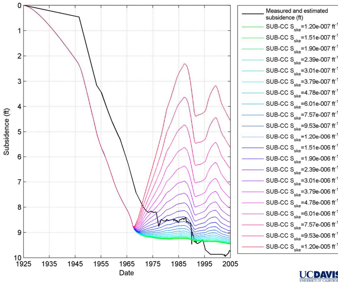
**Figure 70** Sub-Corcoran elastic skeletal specific storage compaction trajectories. Hypo-Corcoran, Corcoran and sub-Corcoran  $K'_v$  values are  $7.10E-06$ ,  $1.20E-05$  and  $1.60E-06$  ft/day, respectively. Hypo-Corcoran, Corcoran and sub-Corcoran  $S'_{skv}$  values are  $1.70E-05$ ,  $3.50E-04$  and  $1.30E-05 \text{ ft}^{-1}$ , respectively. Hypo-Corcoran and Corcoran  $S'_{ske}$  values are  $4.00E-06 \text{ ft}^{-1}$ .
