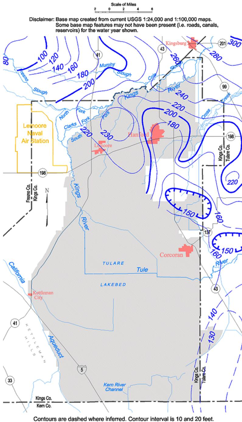
E 27 Unconfined aquifer groundwater contour map, Tulare Lake groundwater basin, Spring 1970.
