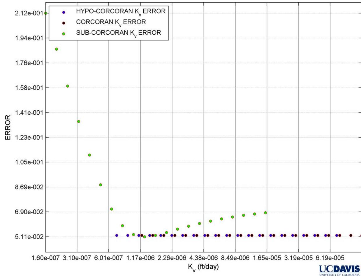
**Figure 71** Vertical hydraulic conductivity error distribution between measured and simulated parameter values. Hypo-Corcoran, Corcoran and sub-Corcoran  $S'_{skv}$  values are 1.70E-05, 3.50E-04 and 1.30E-05  $\text{ft}^{-1}$ , respectively. Hypo-Corcoran, Corcoran and sub-Corcoran  $S'_{ske}$  values are 4.00E-06, 4.00E-06 and 1.20E-06  $\text{ft}^{-1}$ , respectively.
